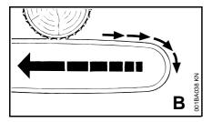
Pushback occurs when the chain on the top of the bar is suddenly stopped when it is pinched, caught or encounters a foreign object in the wood. The reaction of the chain may drive the saw rapidely straight back toward the operator and may cause loss of saw control. Pushback frequently occurs when the top of the bar is used for cutting.
