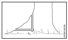
If the tree has large buttress roots, cut into the largest buttress vertically first (horizontally next) and remove the resulting piece.
