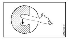
Enlarge the plunge cut as shown in the illustration.
